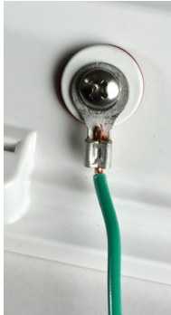
Figure 2.3 - Grounding Lug on SmartSensor V
