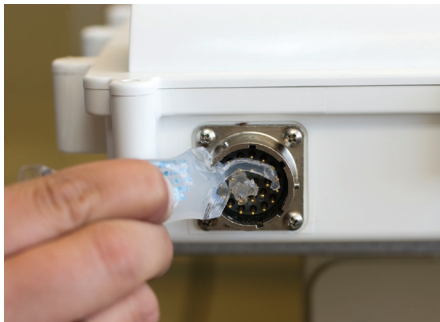
Figure 1.5 – Applying Silicon Dielectric Compound
