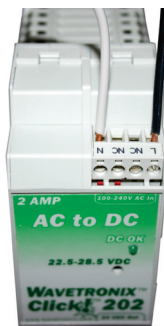
Figure 2.5 – Wiring AC Power into the Click 201/202
