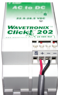
Figure 2.6 – Wiring DC Power Out of the Click 201/202
