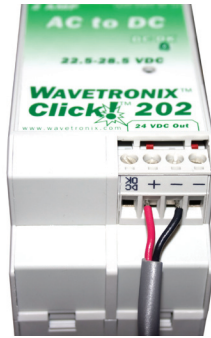
Figure 2.7 – Wiring DC Power Out of the Click 201/202
