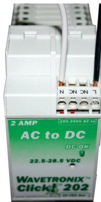
Figure 2.6 – Wiring AC Power into the Click 201/202
