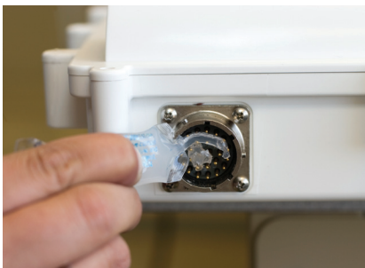
Figure 1.6 – Applying Silicon Dielectric Compound
