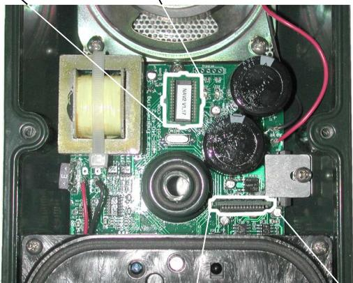
Match polarity dot on Voice Chip with dot on Main PCB (IC should face down).
