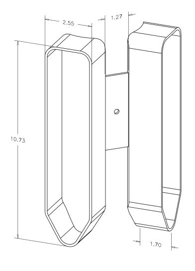
This spacer is designed to offset two Push Button Frames on a 4.5" diameter pole so that two 9" x 12" signs can be mounted without conflict. One spacer is used to mount two Push Button Frames. The spacer is held to the pole by a bolt in the center and the frames mount to the pole with 3" long bolts through the spacer.
