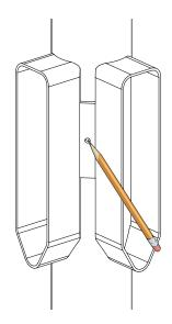
Hold bracket on pole at height and location where you want Push Button Frames positioned. Mark on pole the location of the center hole in the bracket.
