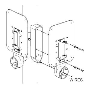
Mount bracket to pole using 1" long 1/4-20 bolt and washer (provided). Route button wires through wire holes, then through the frame holes. Bolt frames to pole using 3" long 1/4-20 bolts and washers (provided).
