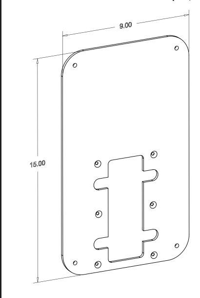
Polara Engineering's 9" x 15" Push Button Frame Adapter is designed to be attached to Polara's PBF5X7-X Push Button Frame, for mounting 9" x 15" crosswalk signs. These adapters can also be used on 2 wire and 4 wire Navigators. Their cast aluminum structure and powder coat finish provides a very strong and attractive mount for crosswalk signs.
