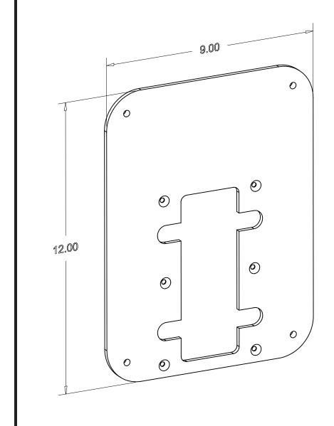
Polara Engineering's 9" x 12" Push Button Frame Adapter is designed to be attached to Polara's PBF5X7-X Push Button Frame, for mounting 9" x 12" crosswalk signs. These adapters can also be used on 2 wire and 4 wire Navigators. Their cast aluminum structure and powder coat finish provides a very strong and attractive mount for crosswalk signs.
