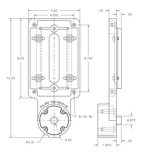
Polara Engineering's Push Button Frames are designed to mount on a 2½" diameter pole up to a 24" diameter pole, or a flat surface. Their cast aluminum structure and powder coated finish provides a very strong and attractive mount for a pedestrian push button and sign.
