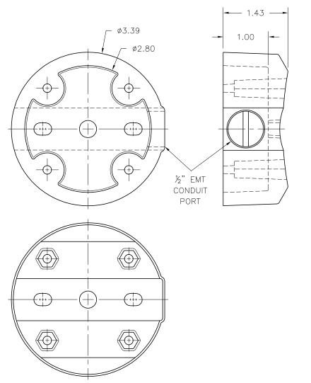
This cast aluminum Button Cup is designed to provide a very strong and semi-low profile mount for Polara's Bulldog Push Button. With Polara's Bulldog Button attached to this mount, the main body of the button extends only approximately 2 inches from the pole. This low profile provides very little foot mount for kids who like to use buttons as a foothold to climb poles; and it is a very rugged answer to vandals who try to damage buttons. Each cup comes with a ½" EMT threaded/plugged conduit port.
